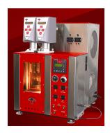
In addition to many other low-temperature tests, the SB+2® multi-purpose bath now has added the capability to run the Freeze-Point (D2386) test method. This method determines the freeze-point of aviation turbine fuels and aviation gasoline where solid hydrocarbon crystals may form. These crystals can restrict the flow of fuel through filters when present in an aircraft's fuel system.
