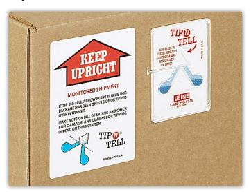
We are now including "Tip N Tell" tilt indicators and/or "Shock Watch" impact stickers on all crated shipments. These visual indicators show if the crate has been tipped over or dropped in transit, and remain unaffected by movement during normal handling conditions. Make sure to check these indicators upon receipt of your shipment and record suspected damage onto your freight carriers receipt prior to signing and accepting the order.
