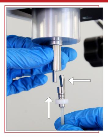
SimAir<sup>®</sup> Quick Connectors are included with the purchase of both the Scanning Brookfield PlusTwo (SB+2) D2983 Insert Module and the SimAir<sup>®</sup> Test Cell Assembly. The Coupling Top and Sleeve are provided with the module purchase, and the Coupling Bottom is included with the SimAir<sup>®</sup> Spindle.
